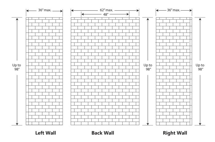
FEATURES Dimensional Tolerance  $\pm \frac{1}{4}$ ". Dimensions needed for site preparation should be measured from the unit. American Bath Group assumes no responsibility for preparatory work.
