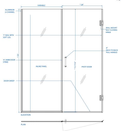
\*NOTE: These measurements are based on a standard 60"x78" enclosure. Heights and Widths are variable and can be ordered to fit specific project requirements.
