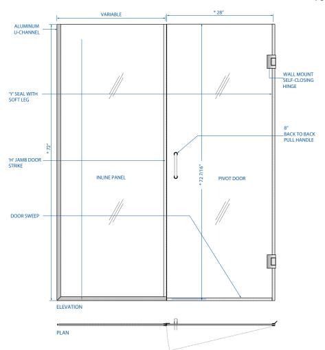
\*NOTE: These measurements are based on a standard 60"x78" enclosure. Heights and Widths are variable and can be ordered to fit specific project requirements.
