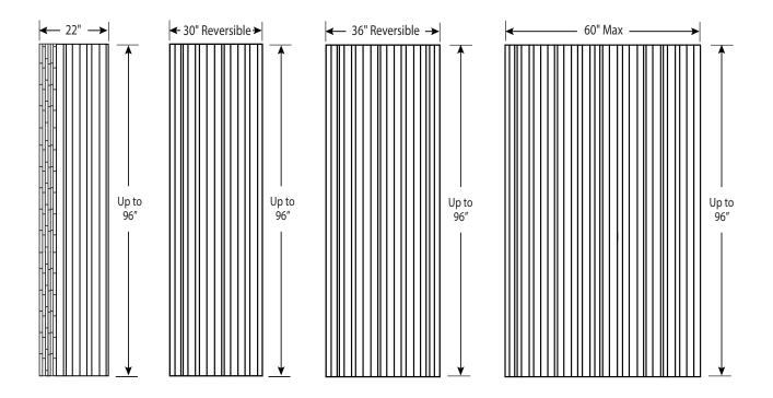
FEATURES Dimensional Tolerance ± 1/4". Dimensions needed for site preparation should be measured from the unit. American Bath Group assumes no responsibility for preparatory work.
