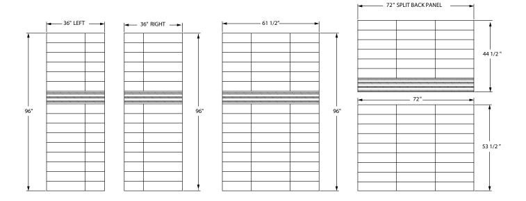
$FEATURES \ \ Dimensional\ Tolerance \pm \ ^{1/4}"\ . \ Dimensions\ needed\ for\ site\ preparation\ should\ be\ measured\ from\ the\ unit.\ American\ Bath\ Group\ assumes\ no\ responsibility\ for\ preparatory\ work.$
