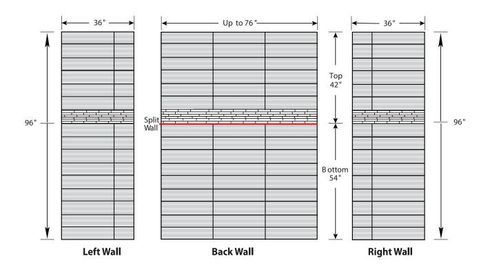
FEATURES Dimensional Tolerance ±<sup>1/4</sup>". Dimensions needed for site preparation should be measured from the unit. American Bath Group assumes no responsibility for preparatory work.
