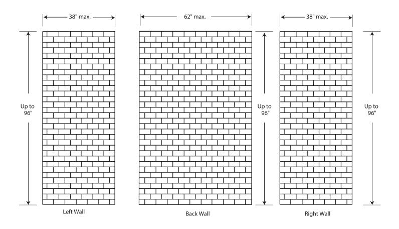
$FEATURES \ \ Dimensional\ Tolerance\ \pm^{1/4}"\ .$  Dimensions needed for site preparation should be measured from the unit. American Bath Group assumes no responsibility for preparatory work.
