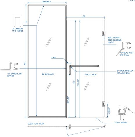
\*NOTE: These measurements are based on a standard 60" x 78" enclosure. Heights and Widths are variable and can be ordered to fit specific project requirements.
