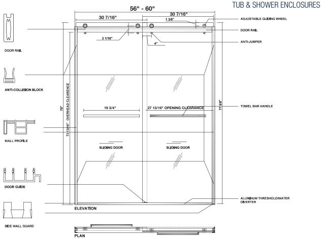
\*NOTE: These measurements are based on a standard 60"x78" enclosure. Heights and Widths are variable and can be ordered to fit specific project requirements.
