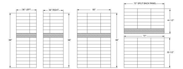
FEATURES Dimensional Tolerance ± 1/6". Dimensions needed for site preparation should be measured from the unit. American Bath Group assumes no responsibility for preparatory work.
