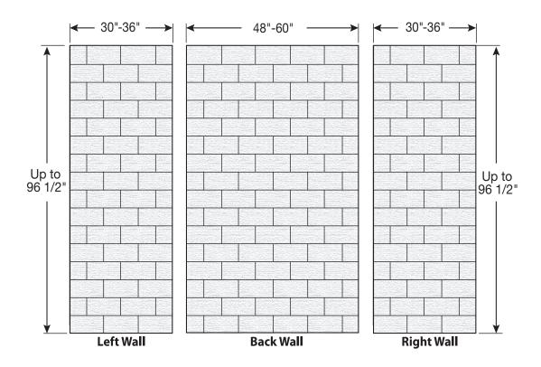
$\textbf{FEATURES} \ \ \text{Dimensional Tolerance} \ \pm \ \textbf{1/6}". \ \ \text{Dimensions needed for site preparation should be measured from the unit. American Bath Group assumes no responsibility for preparatory work.$
