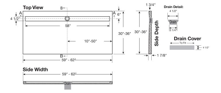
FEATURES Dimensional Tolerance ± 1/8". Dimensions needed for site preparation should be measured from the unit. American Bath Group assumes no responsibility for preparatory work.
