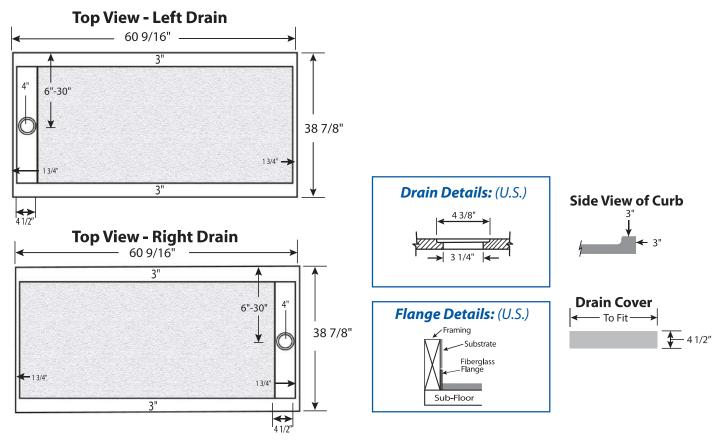
FEATURES Dimensional Tolerance ± 1/6". Dimensions needed for site preparation should be measured from the unit. American Bath Group assumes no responsibility for preparatory work.
