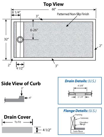
FEATURES Dimensional Tolerance ± 1/6". Dimensions needed for site preparation should be measured from the unit. American Bath Group assumes no responsibility for preparatory work.
