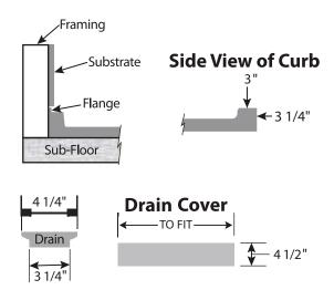
FEATURES Dimensional Tolerance ± 1/8". Dimensions needed for site preparation should be measured from the unit. American Bath Group assumes no responsibility for preparatory work.
