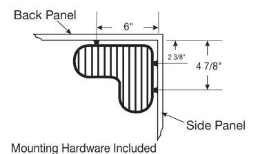
Note: Drill locations in dish may vary so check each dish before drilling. Add a dab of 100% silicone into screw holes under chrome screw cap.
