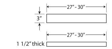
FEATURES Dimensional Tolerance ± 1/6". Dimensions needed for site preparation should be measured from the unit. American Bath Group assumes no responsibility for preparatory work.
