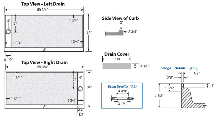
FEATURES Dimensional Tolerance ± 1/6". Dimensions needed for site preparation should be measured from the unit. American Bath Group assumes no responsibility for preparatory work.
