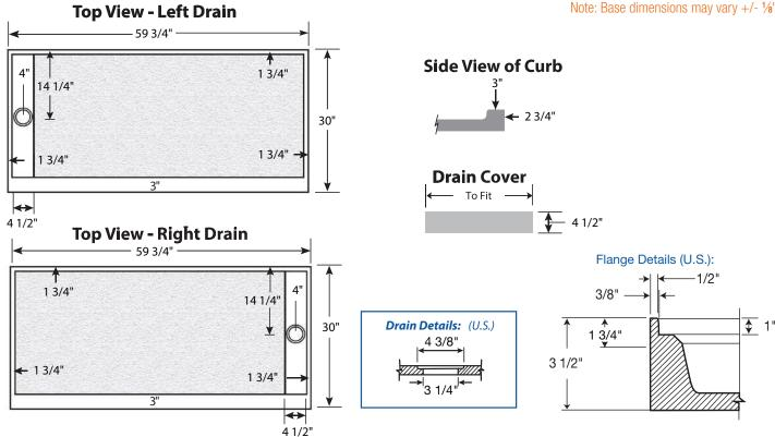
FEATURES Dimensional Tolerance ± 1/8". Dimensions needed for site preparation should be measured from the unit. American Bath Group assumes no responsibility for preparatory work.
