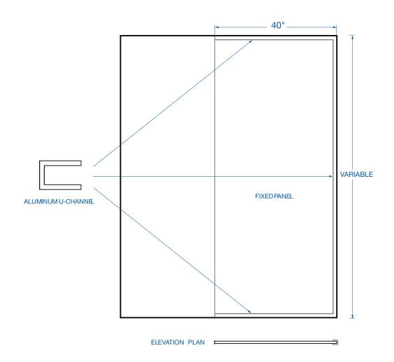
\*NOTE: These measurements are based on a standard 40" x 96" enclosure. Heights and Widths are variable and can be ordered to fit specific project requirements.
