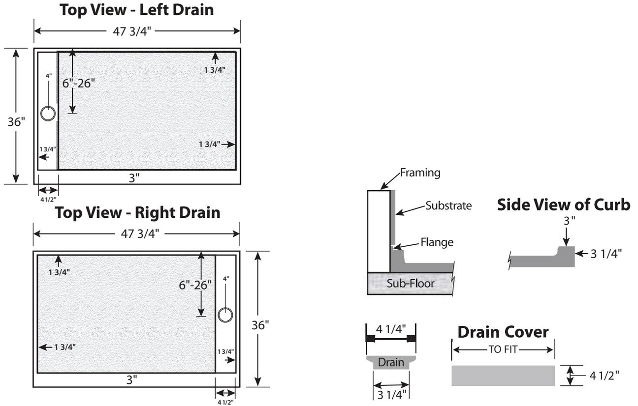
**FEATURES** Dimensional Tolerance  $\pm 1/8"$ . Dimensions needed for site preparation should be measured from the unit. American Bath Group assumes no responsibility for preparatory work.
